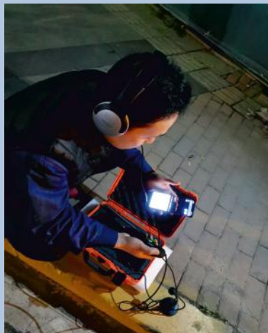
Detect leaks in pipes below floors.
